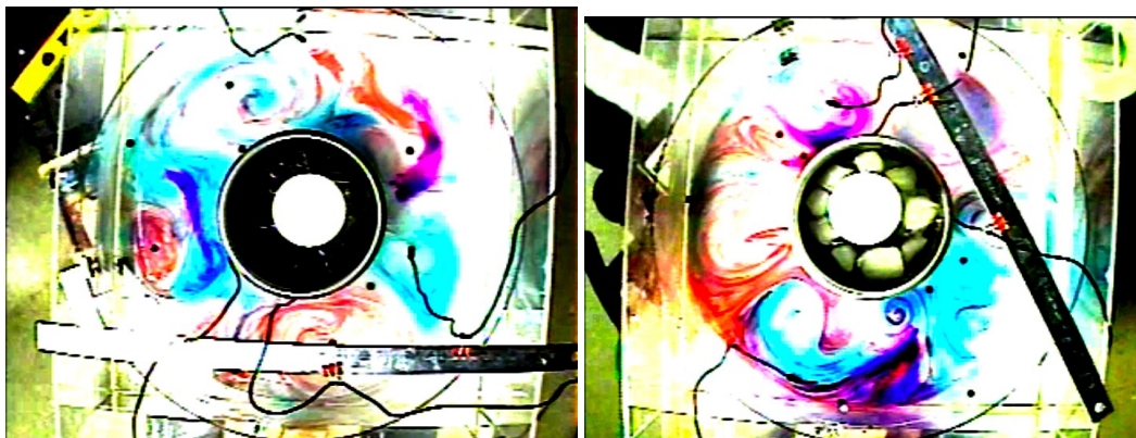
Figure 4. Observed eddy flow patterns in the 5 RPM experiment (left) and 10 RPM experiment (right).
