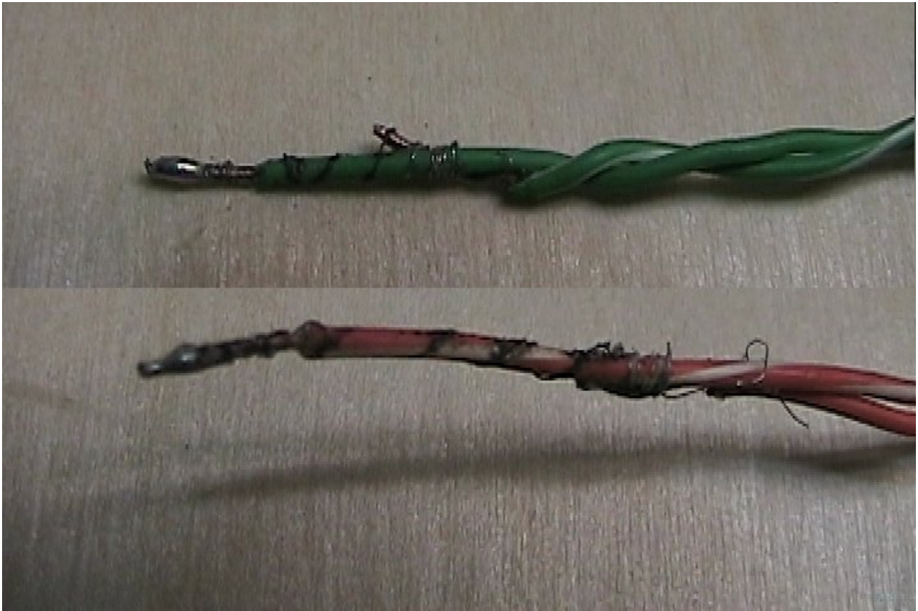
Here's two e-matches that failed.
