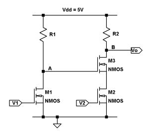
(a) [4 Points] What should be the value of  $R_1$  so that the noise margin at node A is 0.5V?
