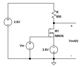
(A) [5 Points] The transfer characteristics of this amplifier can be obtained by sweeping the input voltage between -2.5V and 2.5V. To do so, apply a sine wave at the input with a frequency of 100Hz, an amplitude of 2.5V and an offset of 0V. At the output, appropriately configure the oscilloscope to see at least one full period of the output signal
