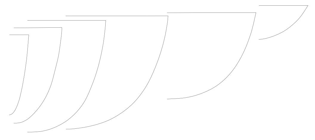
sensor locations from bow to stern (x/L, reference to the deck): 0.05, 0.1, 0.1375, 0.175, 0.525, 0.575, 0.625, 0.675, 0.725, 0.775 profile locations (from left to right): 0.05, 0.1375, 0.275, 0.525, 0.775, 1.0
