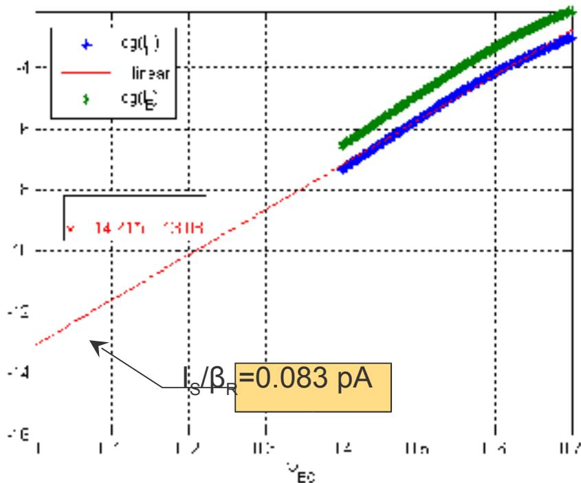
$$\beta_R = 4.18 \rightarrow \alpha_R = \frac{\beta_R}{1 + \beta_R} = 0.807 \rightarrow I_{CS} = \frac{I_S}{\alpha_R} = 0.43 \text{ pA}$$
