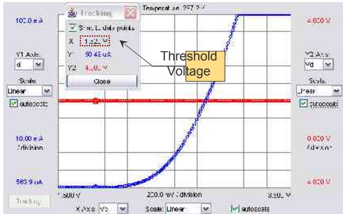
$$\text{Assuming } \frac{W}{L} = \frac{46.5}{1.5} \rightarrow \mu_n C_{ox} = \frac{2LI_{Dsat}}{W(V_{GS} - V_T)^2} = 1.28 \text{ mA/V}^2$$
